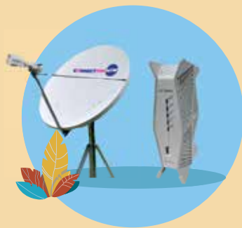
Very Small Aperture Terminal (VSAT)
